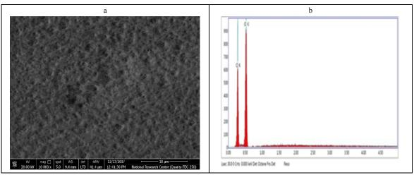
Figure 1. SEM image (a), with EDS spectra (b) for the polycarbonate filter (blank) before sampling.
