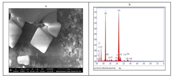
Figure 6. SEM image of sodium chloride particle (a) and its EDX spectra (b) in TPM samples.
