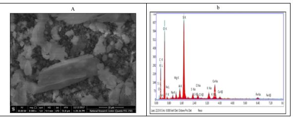
Figure 4. SEM image of Aluminium silicate particles (a) and EDS spectra (b) in TPM samples.
